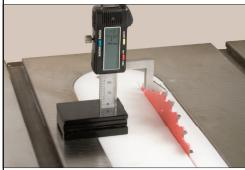
Set the gauge to your desired height and lock into position with the locking knob. Place the digital height gauge next to the saw blade with the foot directly above the blade. Raise the blade until it just touches the base of the foot.
