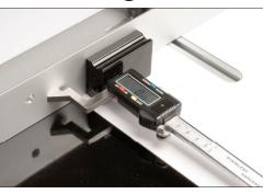
With the digital height gauge placed horizontally on your router table top and up against the fence, slide the foot until it touches the router table fence surface. Press the zero button and the readout should read all zero's.
