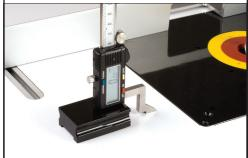
With the digital height gauge placed on your router table top, slide the foot down until it touches the table top surface. Press the zero button and the readout should read all zero's.
