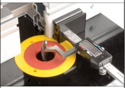
Set the gauge to your desired router bit distance from your fence and lock into position with the locking knob. Place the gauge horizontally on your router table top and up against the fence. Adjust the fence so the foot just touches the desired point on your router bit.
