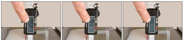
Once you have your measurements made you can easily convert your increments on the readout display by pushing the in/mm/fractions button. This button allows you to toggle between inches, millimeters and fractions.
