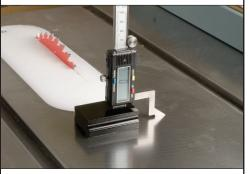
With the digital height gauge placed on your table saw top, slide the foot down until it touches the table top surface. Press the zero button and the readout should read all zero's. ...Using Router Table
