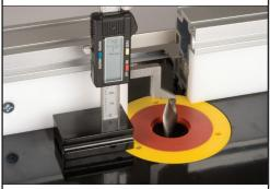
Set the gauge to your desired height and lock into position with the locking knob. Place the digital height gauge next to the router bit with the foot directly above the bit. Raise the bit until it just touches the base of the foot.
